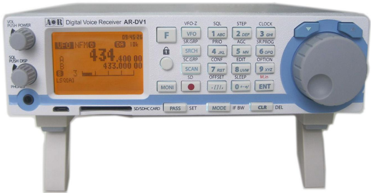
Fig. 1: front view of the AR-DV1. Note the micro-USB and SD/SHDC card sockets. Like many radios (for example the Realistic Pro 2006) it has folding feet. This allows it to present at a good viewing angle whether on a desk or a shelf. Vehicle mounting is often a challenge nowadays as few modern vehicles have any space spare in the dashboard.
