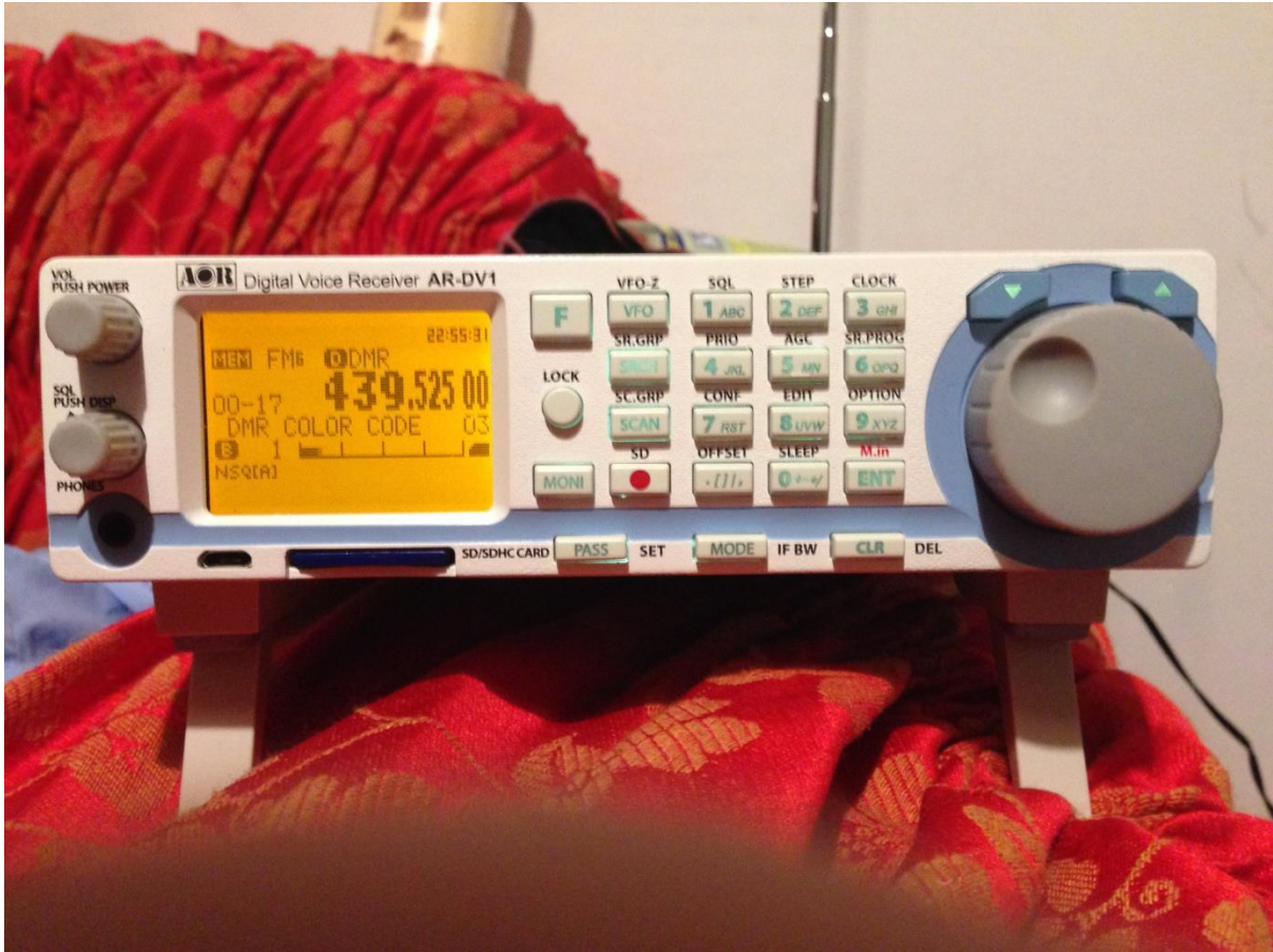
The AR-DV1 now displays the DMR colour code in use when receiving a transmission.
